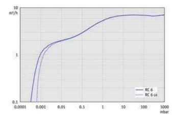
RC 6 - Pump down graph at 60 Hz (10 I volume)
