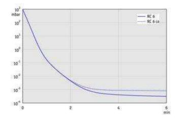
RC 6 - Pumping speed graph at 60 Hz
