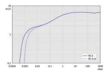
RC 6 - Pump down graph at 50 Hz (10 I volume)
